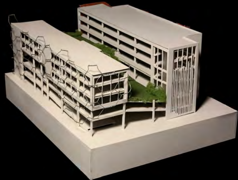
1/8" Scale, Mixed Materials and MDF Board Laser Cut
